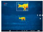
Upon activation Picture in Picture function displays second small image with magnification in the top part of the screen. Small image helps to zoom in on a target while retaining the rest of the field of view visible.
